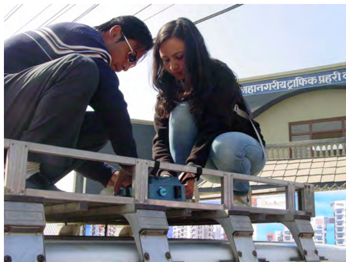
Two students in Dr. Carter's class set up a device to monitor dust at a work facility in Nepal.
