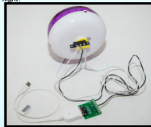
Figure 2. Exercise Wheel with Attached Switch and USB Connector
